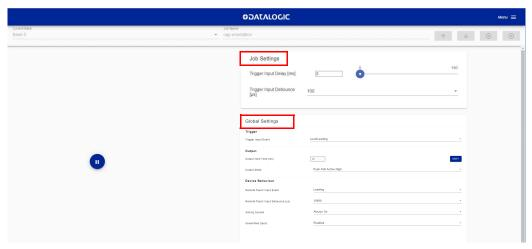
The parameters under <u>Job Settings</u> are variable for each job, which means that any change will only be valid for the current job:
