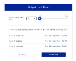
Since the output hold time is a global parameter used by all jobs, the smart-VS shows how the maximum number of objects that can be analyzed by each job present on the device changes as this parameter varies.
