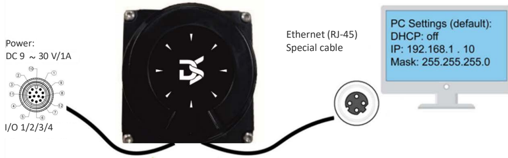
Figure 2 - LGS-A10 Connection
